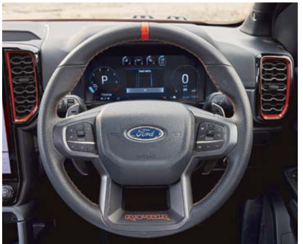
The sports steering wheel has room for a selection of controls including selective drive modes and paddle gear shifters.
